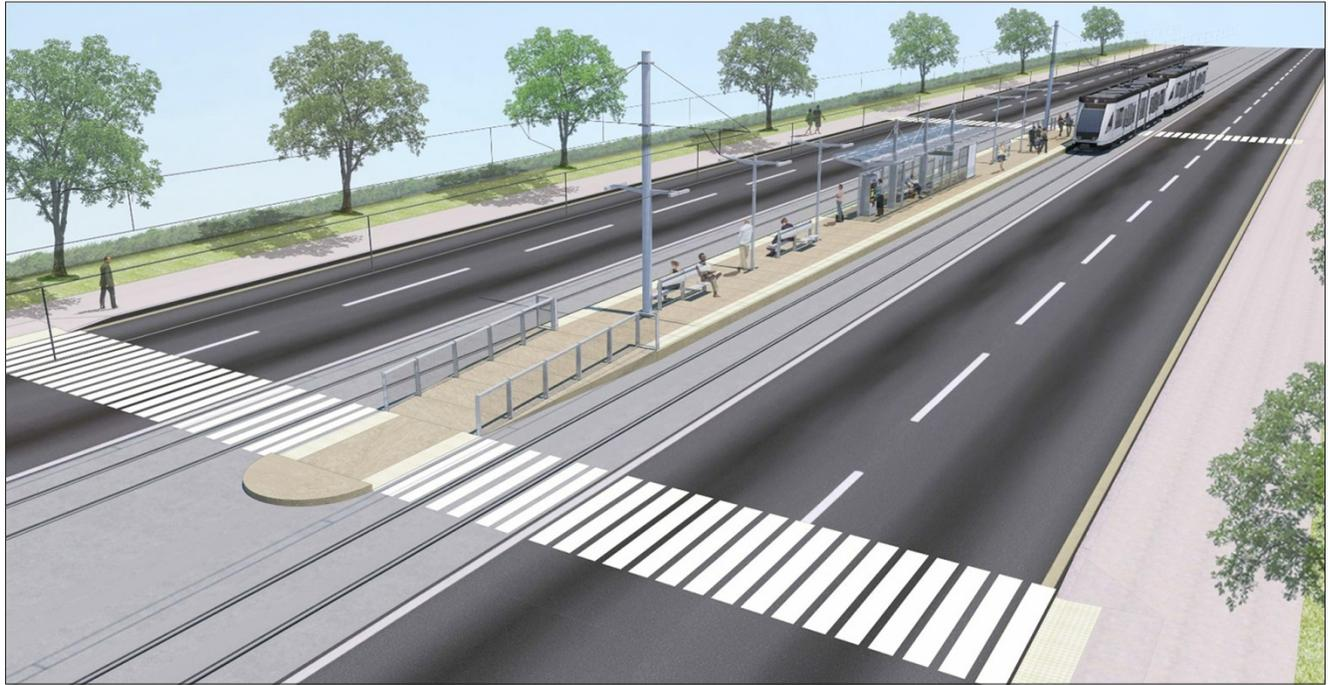
**Figure 1-9. Typical Side Platform Station**
